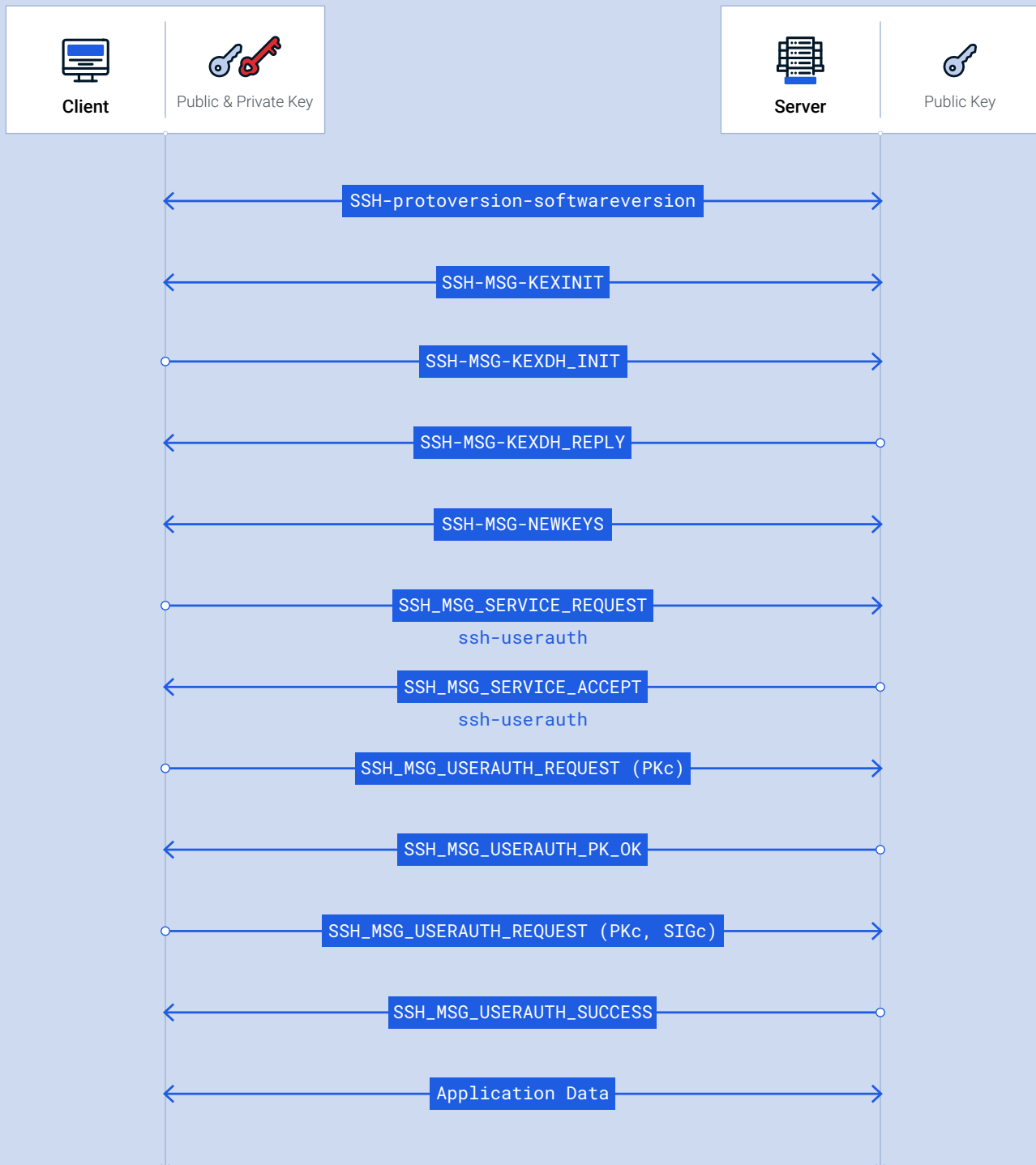
Figure 3.3. SSH Message flow using DH and public key cryptography for user authentication 12
